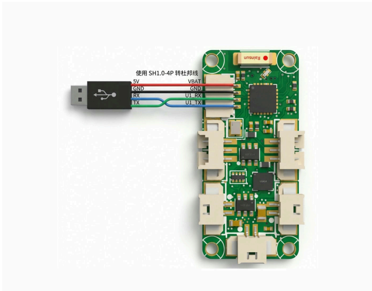
Figure 5: USB-to-TTL wiring to FC UART1
